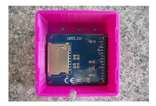
Time to install circuit board, push the end with the 3 push buttons first.
