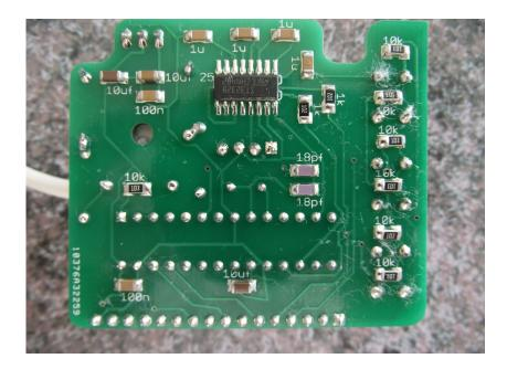
Solder a new wire onto these two pins. Hint, using a long piece of wire makes the job easier.
