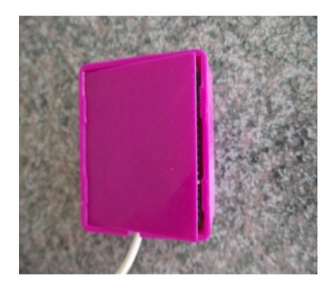
Using a small flat heat screw driver, or if you have long finger nails, stretch the plastic case a bit so the cover can pass through the 4 tabs. If you accidentally damage your plastic case, or want it more solid, you may want to use clear silicone on the back. Silicone is nice in that you can still peel it off should you need access to it the future.
