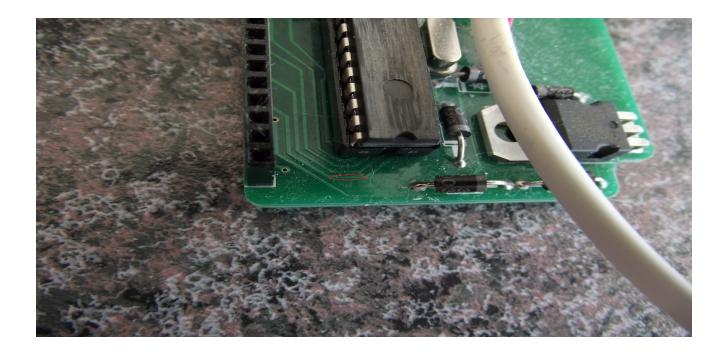
Using a sharp xacto blade or knife, scrape the circuit off. Be careful not to harm the adjacent circuit board traces.
